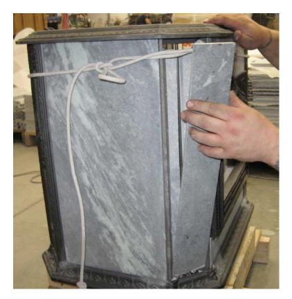
10. Apply a generous amount of furnace cement to the top, beveled edge of the new stone so that there is about a 1/2" of cement where the bevel meets the inside edge of the top frame. This will ensure a proper seal in this area.
