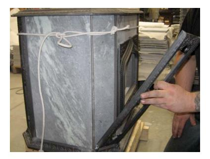
9. Remove the corner stone. Tighten the rope.
