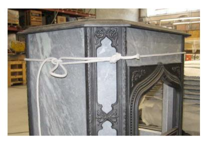
5. Remove the top lid from the stove. This lid is not fastened down and will lift straight up and off.
