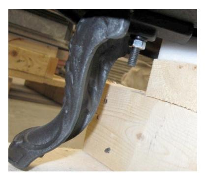
7. Lift the top frame SLOWLY. There will be resistance from the furnace cement and this may take some effort. It may be helpful to use a rubber mallet to gently tap the frame upward. Raise the top frame up just high enough to allow the top edge of the corner cast to be pulled out. It will be necessary to have some slack in the rope to move the corner cast.
